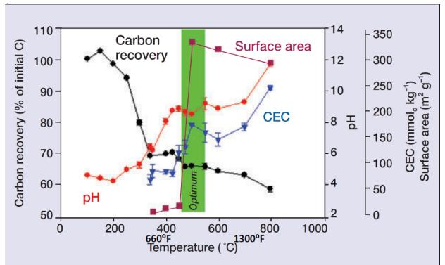
Effect of Pyrolysis Temperature on Biochar Conversion Rate and Product Surface Area
