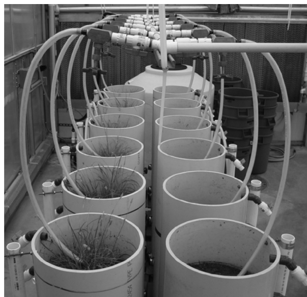
Fig. 1. The two sets of bioretention columns used to filter runoff from the September 2012 storm event. All columns contain a mixed layer of bioretention soil medium overlying a gravel aggregate drainage layer. The columns on the left are planted with Carex flacca .
